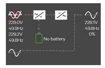
Figure 5-2 Bypass to inverter Mode
