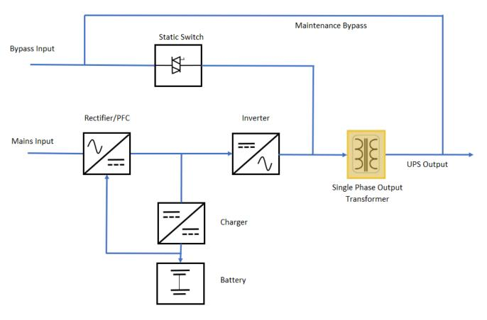
Figure 1-4 UPS Operating Principle
