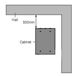
Figure 2-2 Installation Clearances (Top view of rack installation)
