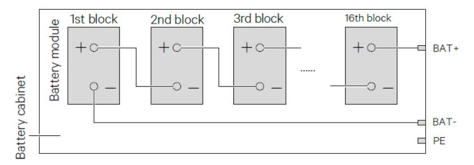
Figure 3-4 Internal connection diagram for positive battery string and negative battery string
