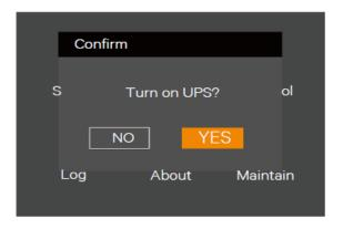
Figure 2-7 Turning on UPS
