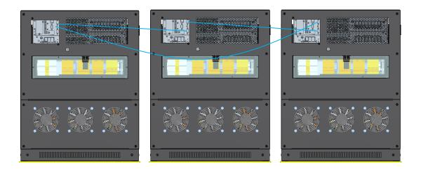
Figure 3-1 Cabel Connection schematic diagram of 2 + 1 parallel system (20kVA)
