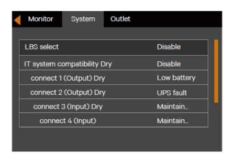
Figure 3-8 LBS Parameter Setting Interface
