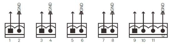
Figure 6-2 Pin layout of dry contact ports
