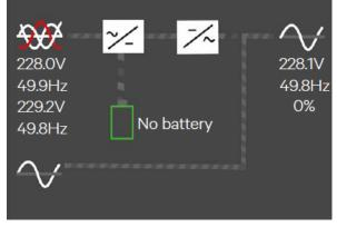
Figure 5-2 Bypass Normal Interface
