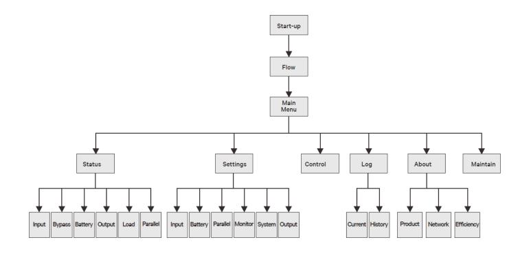
Figure 4-11 LCD Menu Structure
