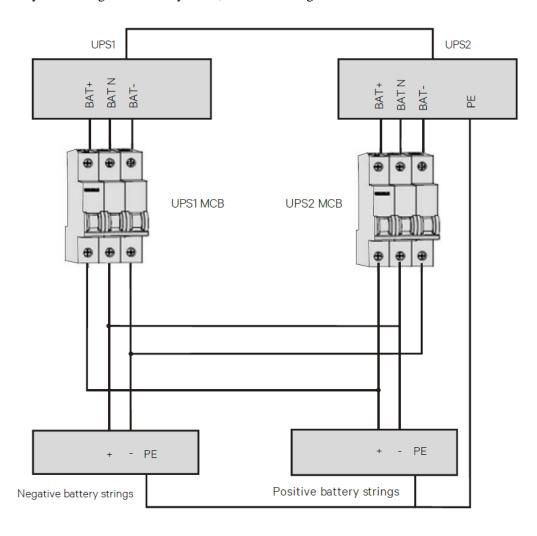
Figure 3-3 Connection diagram fof shared battery string in 1+1 parallel system
