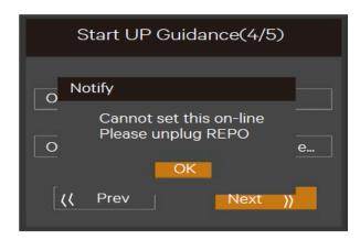
Figure 4-8 Prompt of removing REPO terminal
