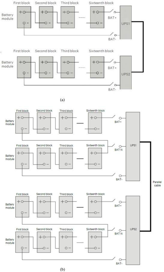
Figure 3-2 Connection Principle Diagram upon using battery string independently in (a) 10kVA and (b) 20kVA respectively
