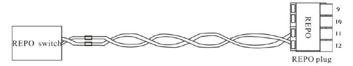
Figure 6-3 Repo cable connection
