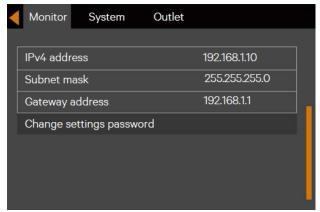
Figure 6-4 Changing UPS Network Parameters
